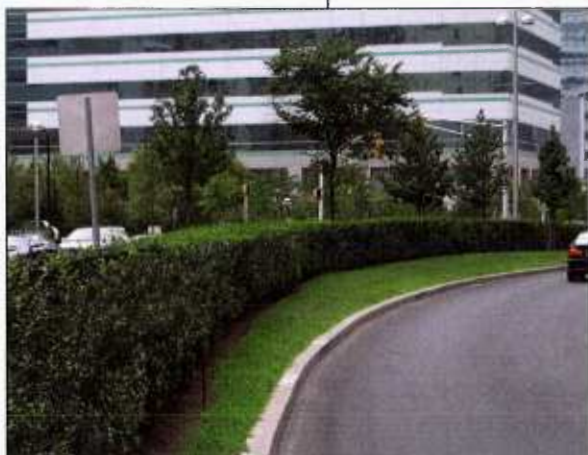
Exhibit 3-34. Median Plantings to Discourage Midblock Crossing (16).
