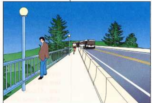
Exhibit 3-12. Bridge with Protective Barrier at Curb (20).
