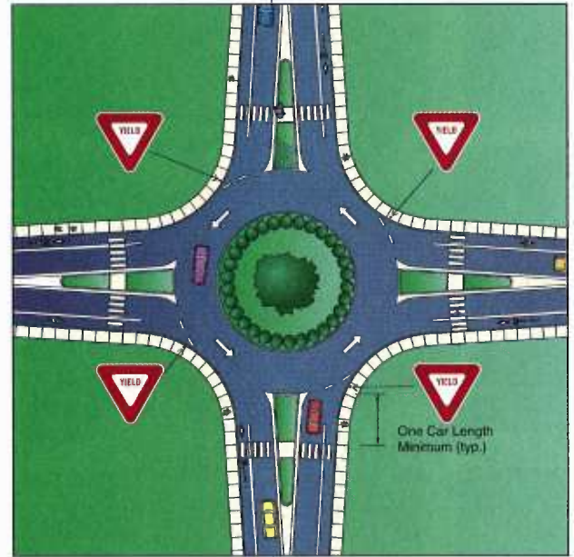
Exhibit 3-23. Modern Roundabout Design (26).
